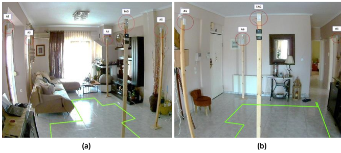
Fig. 5: Anchors placement within the room: (a) A2, A3, A4, A5, (b) A1, A5, A6.
